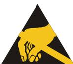
The measuring system contains electrostatically endangered circuit elements and units which can be destroyed by an improper use.
