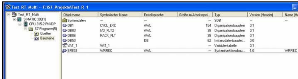
Figure 9: Preset execution by means of the CPU 315-2 PN/DP and SFB53
