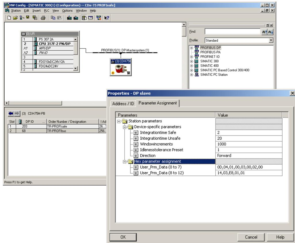
The screenshot shows the SIMATIC Manager HW Config interface. The main window displays a rack configuration with slots 1 through 5. Slot 2 contains a CPU 317F-2 PN/DP. A PROFIBUS DP connection is established between the CPU and a DP slave (CDH75M-PB). The Properties - DP slave dialog box is open, showing the Parameter Assignment tab. The dialog box contains a table of parameters and their values.
