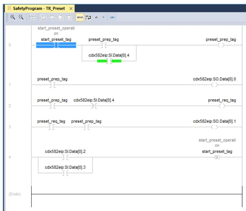
The preset procedure can only be executed if the safe input connection and the safe output connection are configured and established (Executing).
