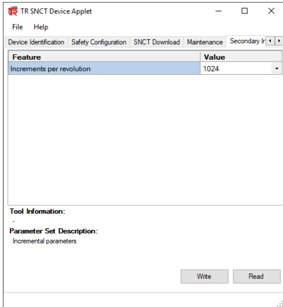
Figure 3: TR SNCT Device Applet: Parameterize second interface
