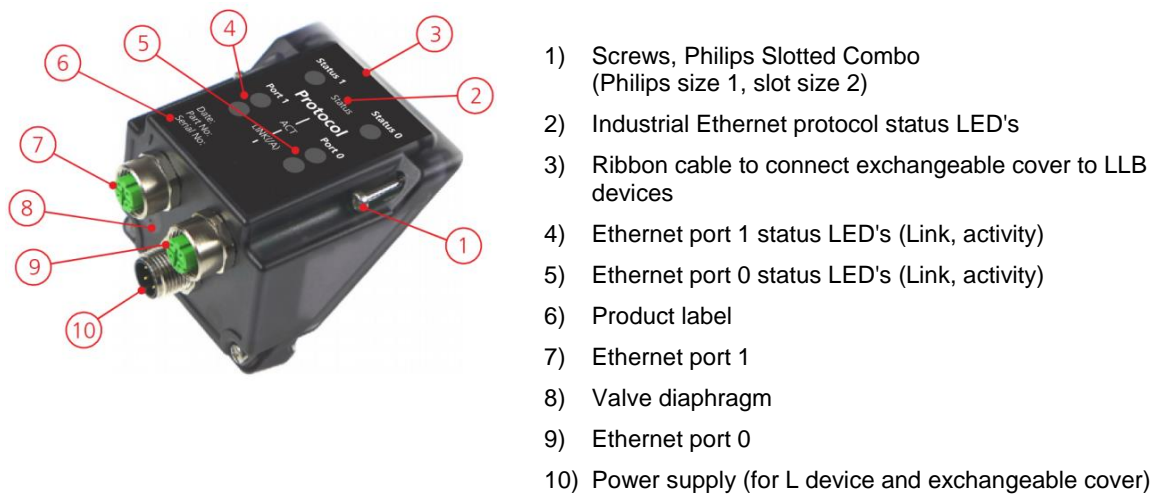
Figure 26: Components with detail information of the exchangeable cover with Industrial Ethernet
