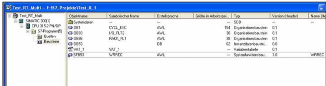
Figure 8: Preset execution by means of the CPU 315-2 PN/DP and SFB53
